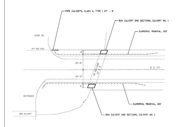
PROPOSED BOX CULVERT END SECTIONS AT SN 095-2481
