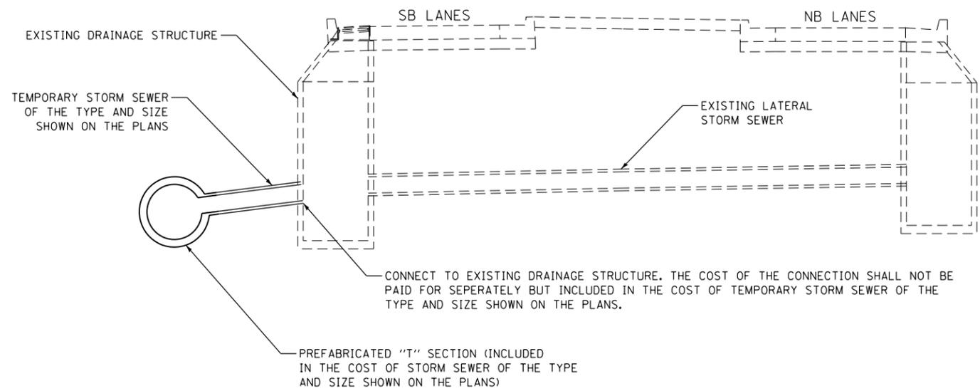
**TEMPORARY STORM SEWER CONNECTION DETAIL**
