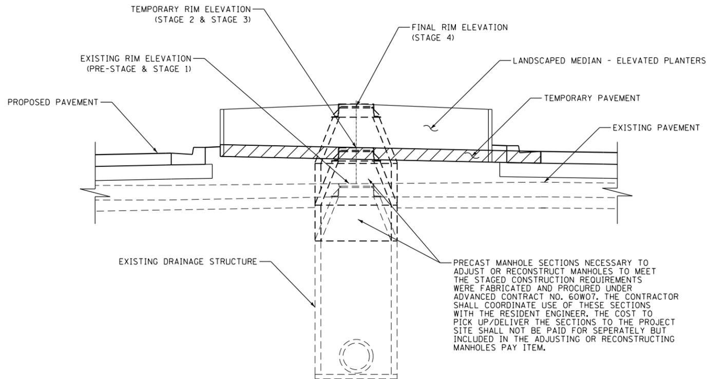
**MEDIAN MANHOLE ADJUSTMENT/RECONSTRUCTION DETAIL**
