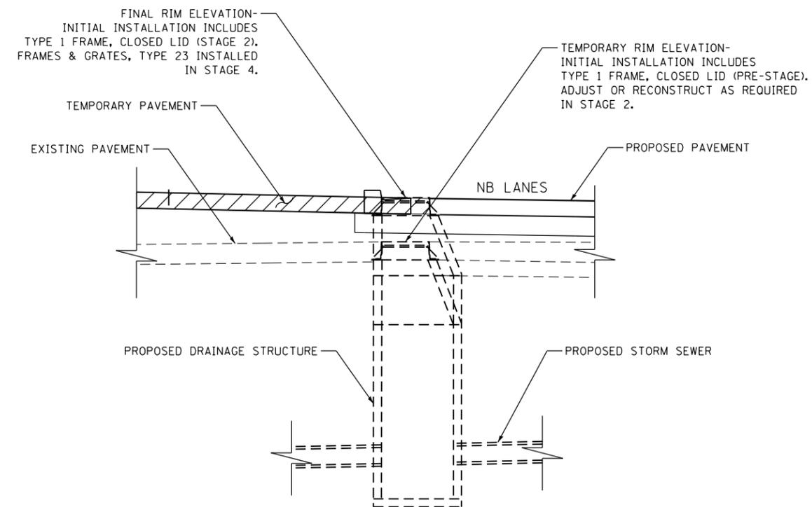
**NB EDGE OF MEDIAN DRAINAGE STRUCTURE ADJUSTMENT/RECONSTRUCTION DETAIL**
