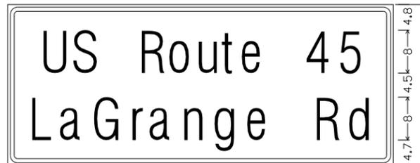
D3-2: 72"x30"; 1.9" Radius, 0.8" Border, 0.5" Indent, Green on Green; [US Route 45] White C 2K; [LaGrange Rd] White D 2K; Table of widths and spaces.
