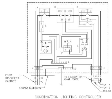
2-1/C \*10 AWG, 600 V TYPE RHW, SOLID COLOR CODED CABLES
