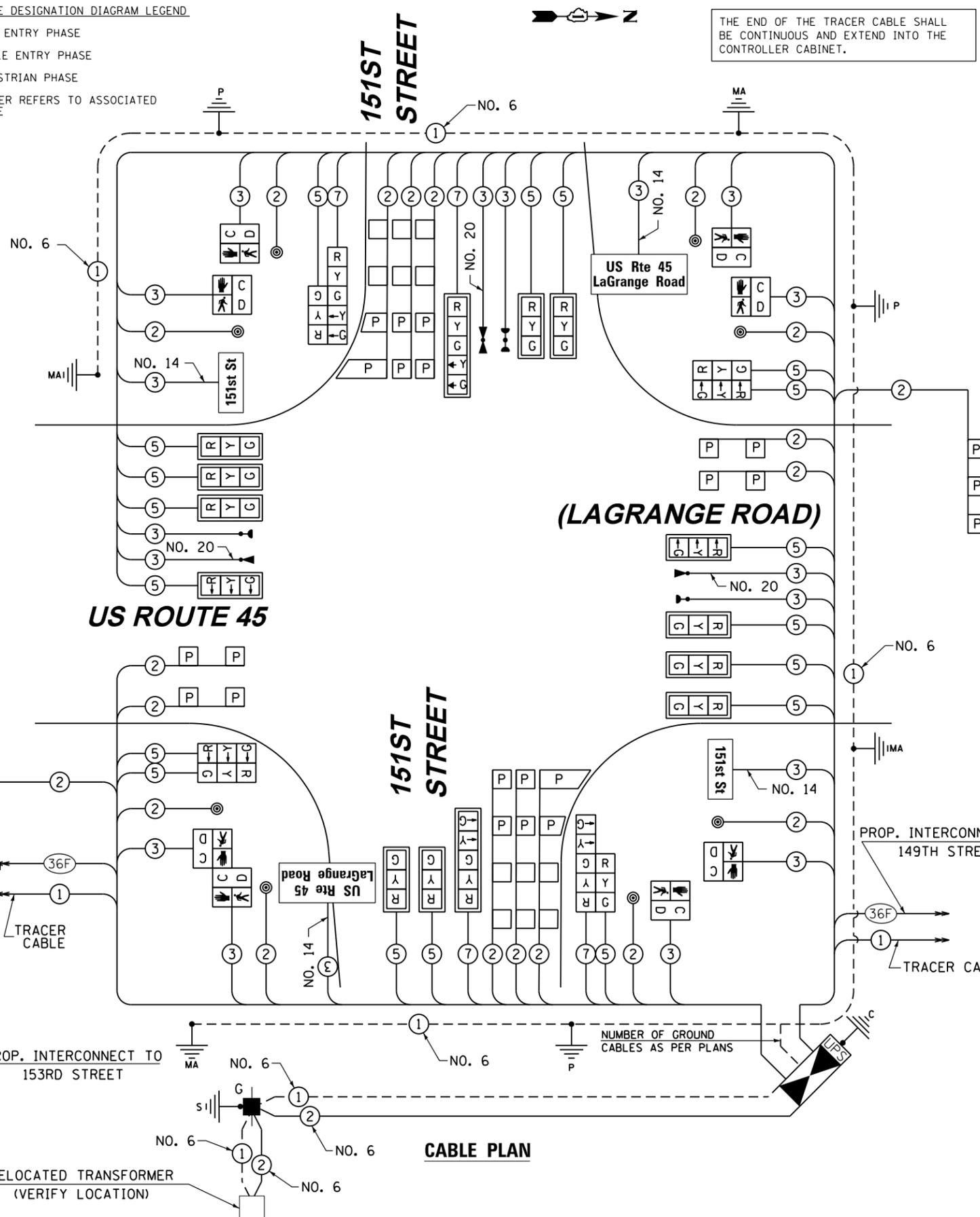
THE END OF THE TRACER CABLE SHALL BE CONTINUOUS AND EXTEND INTO THE CONTROLLER CABINET.
