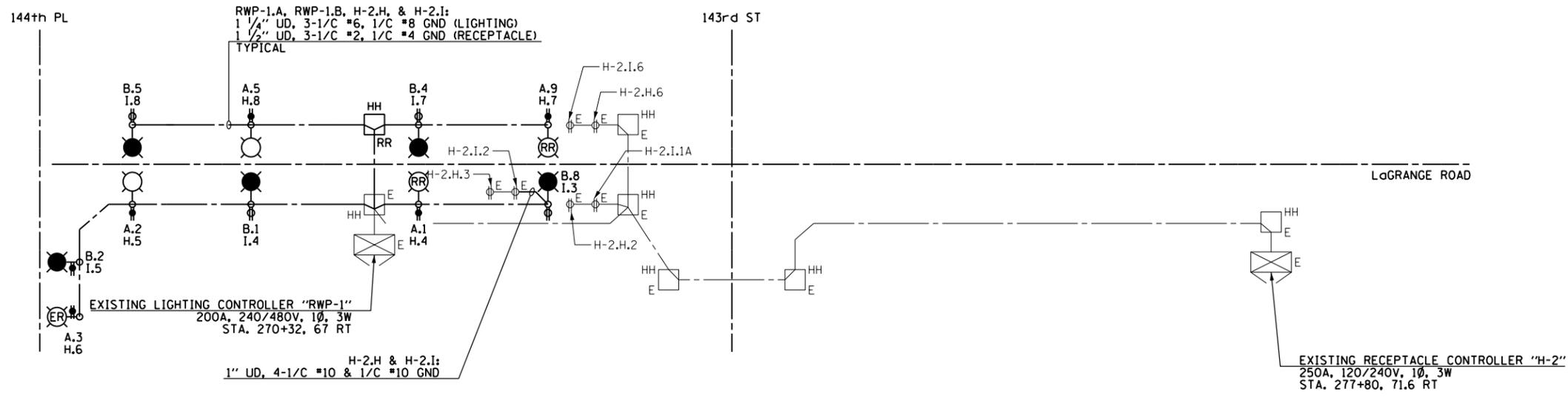
**EXISTING LIGHTING CONTROLLERS "RWP-1" & "H-2" WIRING MODIFICATION DIAGRAM**
