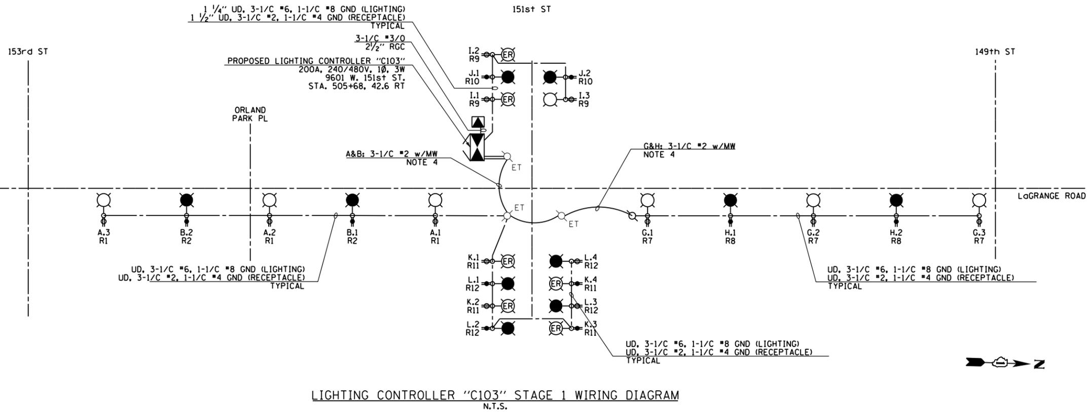
LIGHTING CONTROLLER "C103" STAGE 1 WIRING DIAGRAM
