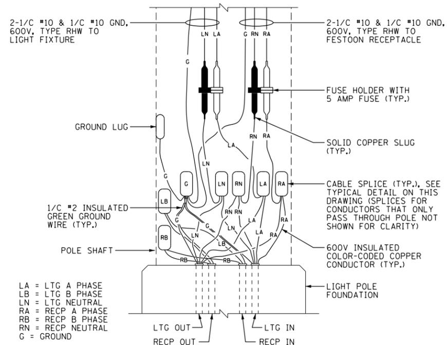
TYPICAL POLE BASE WIRING DETAIL
