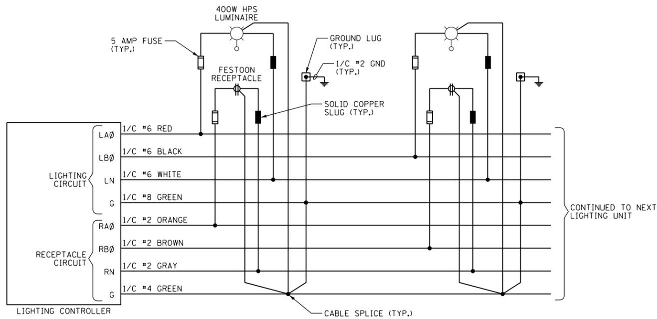
TYPICAL LIGHTING UNIT AND RECEPTACLE WIRING DIAGRAM
