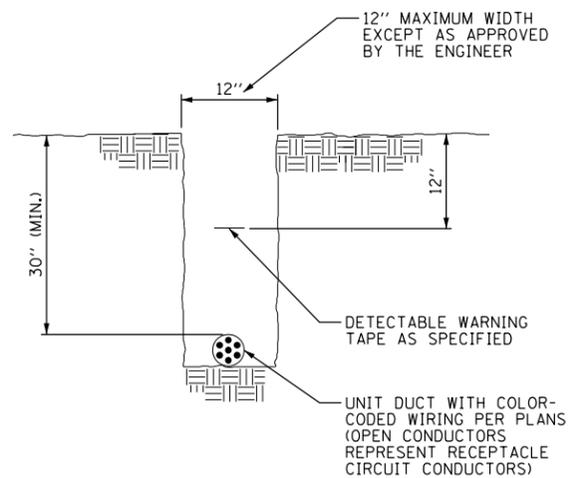
TYPICAL UNIT DUCT IN TRENCH DETAIL
