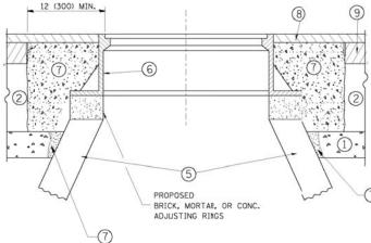
EXISTING BROKEN FRAMES AND LIDS SHALL BE REMOVED AND DISPOSED OF BY THE CONTRACTOR AND SHALL BE REPLACED AS DIRECTED BY THE ENGINEER. REPLACEMENT FRAMES AND LIDS WILL BE PAID FOR IN ACCORDANCE WITH ARTICLE 109.34 OF THE STANDARD SPECIFICATIONS UNLESS A SEPARATE PAY ITEM HAS BEEN PROVIDED.
