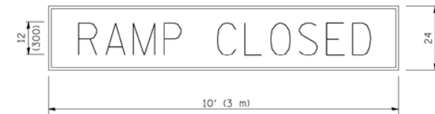
RAMP CLOSURE ADVANCE WARNING SIGN
