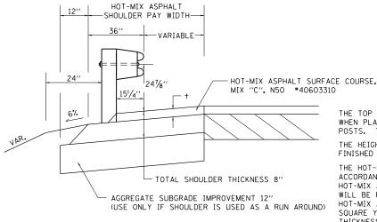
t = SEE TYPICAL SECTIONS FOR THICKNESS
