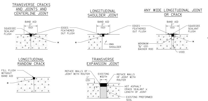
\* HOT ASPHALT CRACK SEALANT
