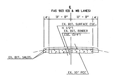
TO BE USED: STA. 195+00 TO STA. 226+45 (SN 100-0040 OMITTED) PROP. CLASS B PATCHES TO BE USED.
