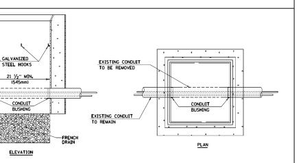
1. HANDHOLE CONSTRUCTED PER STATE STANDARD 814001. 2. REMOVAL OF THE EXISTING CONDUIT FROM THE HANDHOLE AND THE INSTALLATION OF THE CONDUIT BUSHINGS SHALL BE INCLUDED WITH THE COST OF THE HANDHOLE.
