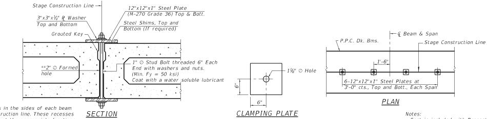
\*\*Cast semi-circular recesses in the sides of each beam adjacent to the stage construction line. These recesses should align to form a hole at the appropriate locations for the clamping device bolts
