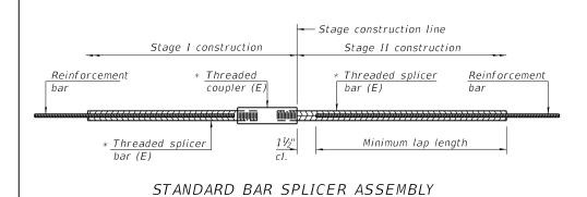
Threaded splicer bar length = min. lap length +  $1\frac{1}{2}$ " + thread length
