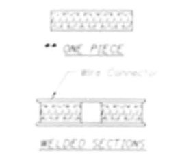
SPLICER ALTERNATIVES Heavy Hex Nuts conforming to ASTM A 563, Grade C, D or L7 may be used.
