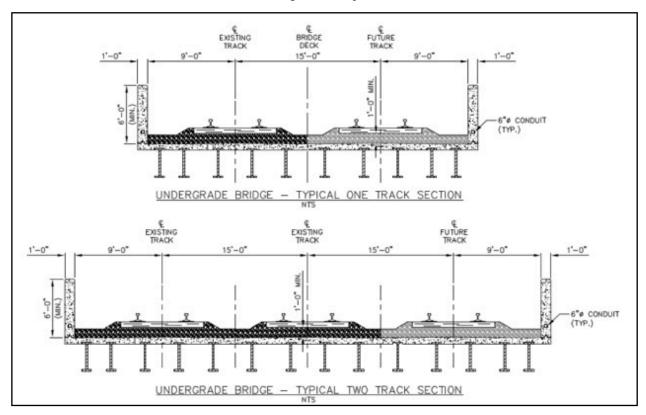
Standard clearances are for tangent track and increases must be provided to account for effects from curvature and superelevation.
