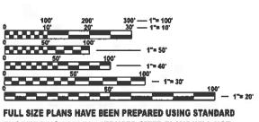
ENGINEERING SCALES. REDUCED SIZED PLANS WILL NOT CONFORM TO STANDARD SCALES. IN MAKING MEASUREMENTS ON REDUCED PLANS, THE ABOVE SCALES MAY BE USED.
