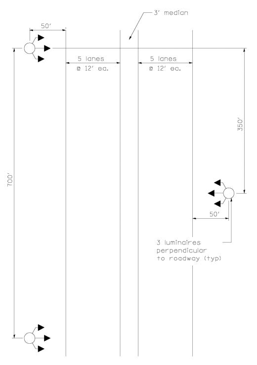
LUMINAIRE ORIENTATION DIAGRAM FOR 750W LUMINAIRES (NOT TO SCALE)
