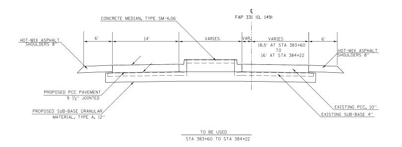
MATCH EXISTING PAVEMENT SLOPES CONCRETE MEDIAN, TYPE SM-4.06 STA 383+60 TO STA 384+22 CONSTRUCT ACCORDING TO STANDARD 606301
