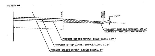
LIMITS OF HOT-MIX ASPHALT SURFACE REMOVAL, BUTT-JOINT SHALL BE FROM EDGE OF PAVEMENT TO RADIUS RETURNS AS SHOWN ABOVE, EXCEPT AT ST. LOUIS STREET WHERE REMOVAL LIMITS SHALL BE 15' FROM EDGE OF PAVEMENT.
