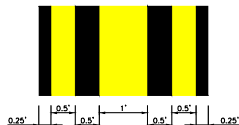
ENLARGEMENT OF ENHANCED MARKING
