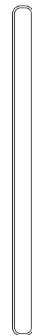
RS PANEL - FLUORESCENT GREEN (RETROREFLECTIVE PANEL) 2" x 84" 1.2 SQ. FT. SIGN PANEL - TYPE 1
