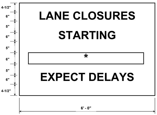
\*CONTRACTOR SHALL PROVIDE DATE FOR START OF LANE CLOSURE AND SHALL ERECT SIGNS A MINIMUM OF ONE (1) WEEK IN ADVANCE OF THE START OF THE WORK.
