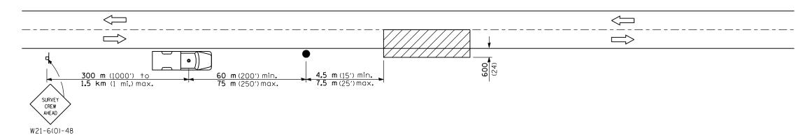
FLAGGER SHALL BE EQUIPPED WITH AND REQUIRED TO USE A HIGH INTENSITY, OR HIGH PERFORMANCE " STOP - SLOW "
