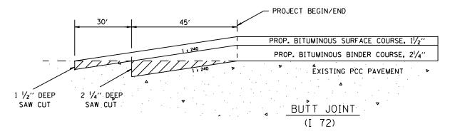
NOTE: TO BE PAID FOR AS PCC SURFACE REMOVAL - BUTT JOINT.
