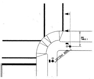
RECOMMENDED PUSHBUTTON LOCATIONS FOR ACCESSIBLE PEDESTRIAN SIGNALS SHALL BE IN ACCORDANCE WITH THE CURRENT MUTCO (SEE NOTE 1). TO MEET MUTCO REQUIREMENTS, PEDESTRIAN SIGNAL PUSHBUTTONS MAY HAVE TO BE
