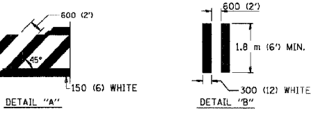
TYPICAL CROSSWALK MARKING
