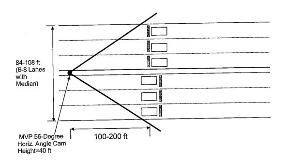
Figure 2. MVP Sensor Adjacent to Lanes of Traffic.
