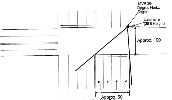
Figure 3. MVP Sensor Location for Optimal Stop Line Detection.
