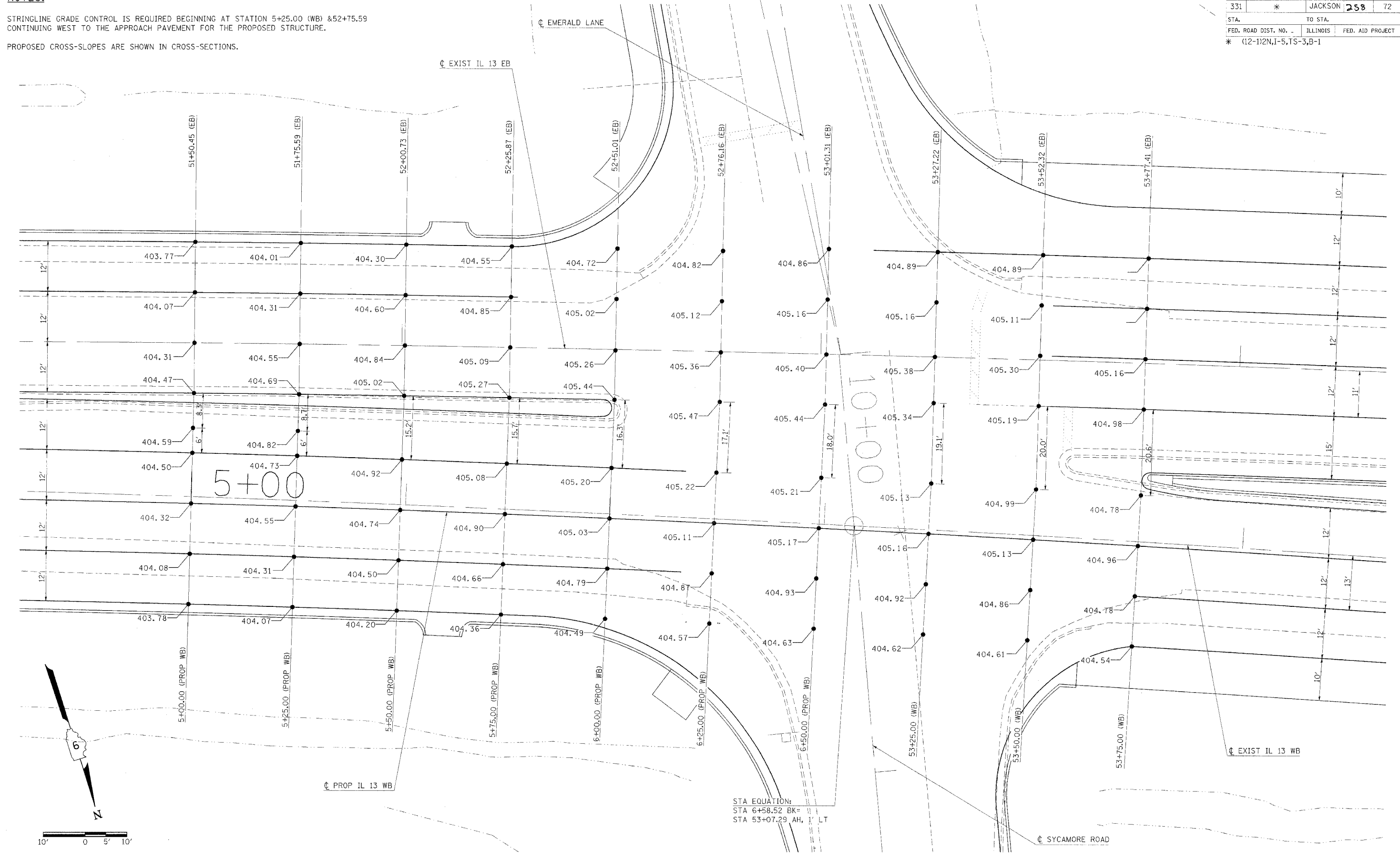
DETAIL : FINAL PAVEMENT ELEVATIONS EMERALD / SYCAMORE INTERSECTION
