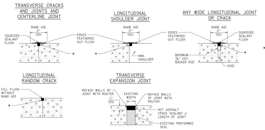
\* HOT ASPHALT CRACK SEALANT
