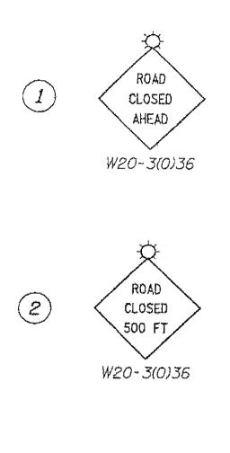
Post mounted sign with Type A Flashing Light
