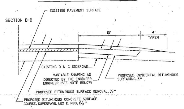
IF EXISTING SUB-BASE IS INADEQUATE; AS DETERMINED BY THE ENGINEER, THE SIDERDADS SHALL BE CORED OUT AND AGGREGATE SUB-BASE, TYPE B SHALL BE PLACED FOR BASE. THE COST OF CORING OUT THE SIDEROAD SHALL BE INCLUDED IN THE COST OF THE AGGREGATE BASE COURSE. IF EXISTING SUB-BASE IS DETERMINED TO BE ADEQUATE, THE AGGREGATE BASE COURSE SHALL BE DELETED AND THE PREPARATION OF THE BASE SHALL BE CONSTRUCTED ACCORDING TO ARTICLE 406.19
