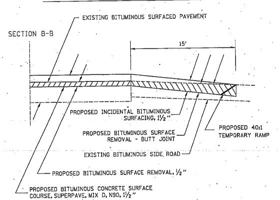
IF EXISTING BASE COURSE IS INADEQUATE, AS DETERMINED BY THE ENGINEER, THE SIDE ROADS SHALL BE CORED OUT AND AGGREGATE BASE COURSE, TYPE B SHALL BE PLACED FOR BASE. THE COST OF CORING OUT THE SIDE ROAD SHALL BE INCLUDED IN THE COST OF THE AGGREGATE BASE COURSE. IF EXISTING BASE COURSE IS DETERMINED TO BE ADEQUATE, THE AGGREGATE BASE COURSE SHALL BE DELETED AND THE PREPARATION OF THE BASE SHALL BE CONSTRUCTED ACCORDING TO ARTICLE 406.19.
