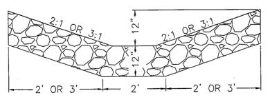
DETAIL OF AGGREGATE DITCH (SPECIAL)
