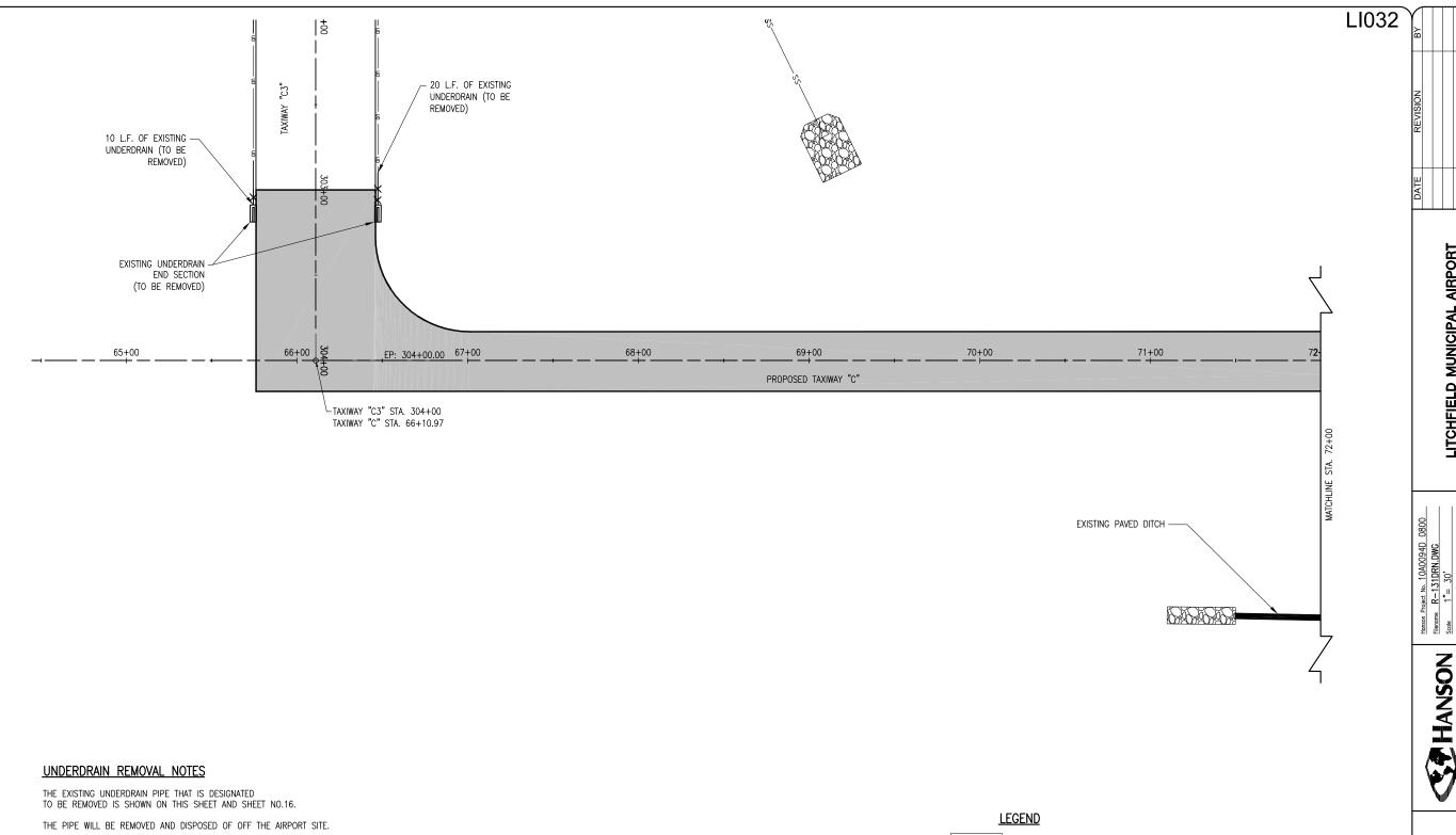
THE CONTRACTOR WILL BACKFILL THE TRENCH WITH THE SELECT EXCAVATED MATERIAL IF THE AREA IS NOT UNDER PROPOSED PAVEMENT. BACKFILL OF AREAS THAT ARE LOCATED UNDER PROPOSED PAVEMENT WILL BE WITH CA-7. THE CA-7 WILL EXTEND TO WITHIN 16" OF THE TOP OF THE PROPOSED SUBGRADE.
