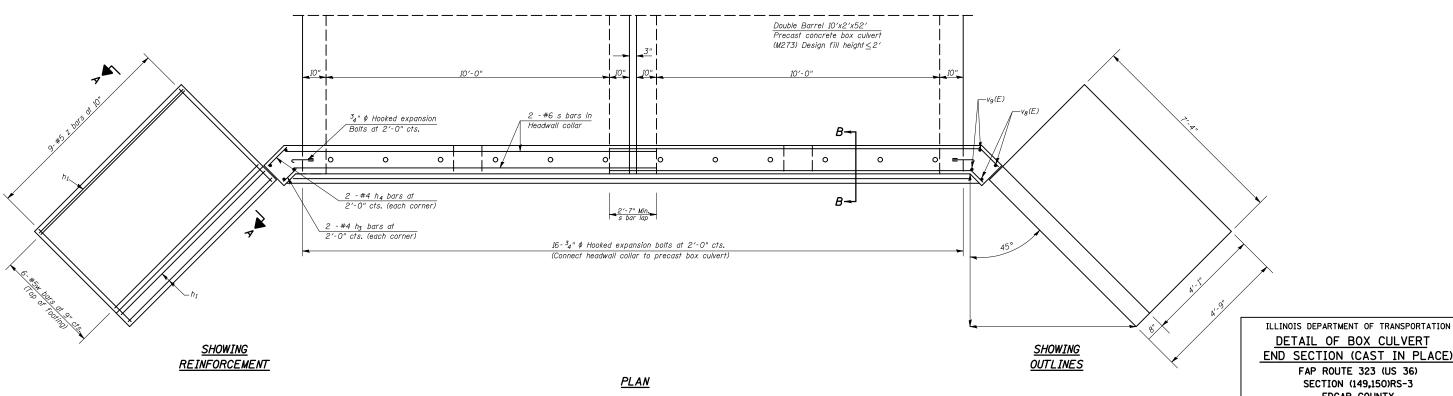
DETAIL OF BOX CULVERT END SECTION (CAST IN PLACE) FAP ROUTE 323 (US 36)
