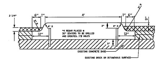
DETAIL OF CONCRETE MEDIAN, TYPE SB, SPECIAL
