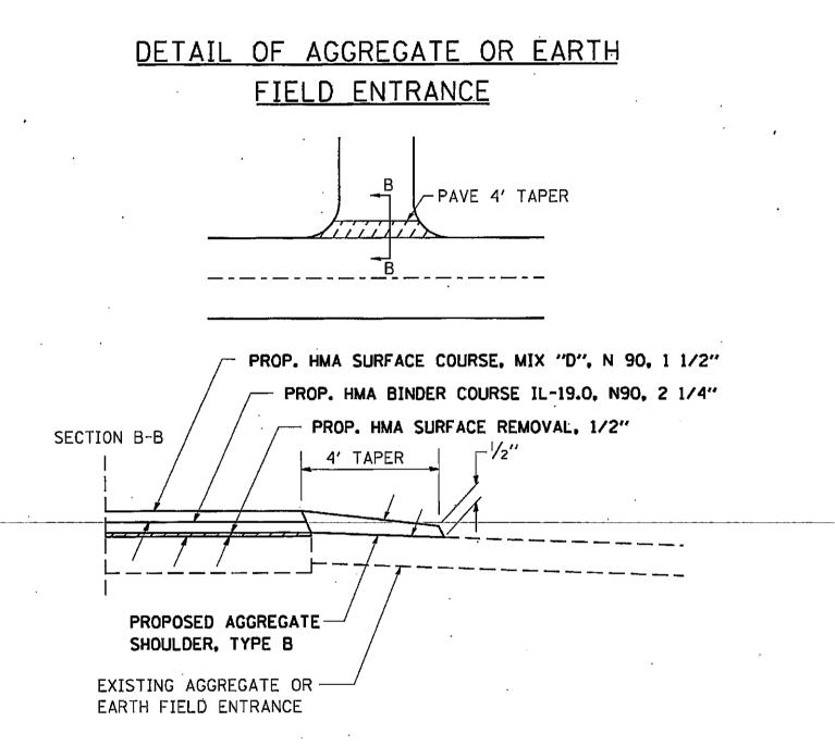
PREPARATION OF EXISTING SURFACE AND ANY EXCAVATION FOR ENTRANCES SHALL BE IN ACCORDANCE WITH ARTICLE 406.09 OF THE STANDARD OF SPECIFICATIONS.
