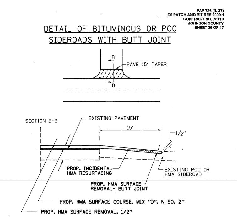
IF EXISTING BASE COURSE IS INADEQUATE, AS DETERMINED BY THE ENGINEER, THE SIDEROADS SHALL BE CORED OUT AND AGGREGATE BASE COURSE, TYPE B SHALL BE PLACED FOR BASE. THE COST OF CORING OUT THE SIDEROAD SHALL BE INCLUDED IN THE COST OF THE AGGREGATE BASE COURSE. IF EXISTING BASE COURSE IS DETERMINED TO BE ADEQUATE, THE AGGREGATE BASE COURSE SHALL BE DELETED AND THE PREPARATION OF THE BASE SHALL BE CONSTRUCTED ACCORDING TO ARTICLE 406.09.
