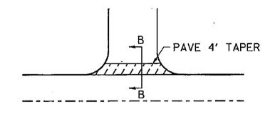
PROP. HMA SURFACE COURSE, MIX "D", N 90, 2" PROP. HMA SURFACE REMOVAL, 1/2" SECTION B-B 4' TAPER 4' TA
