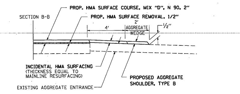
PREPARATION OF EXISTING SURFACE AND ANY EXCAVATION FOR ENTRANCES SHALL BE IN ACCORDANCE WITH ARTICLE 406.09 OF THE STANDARD SPECIFICATIONS.
