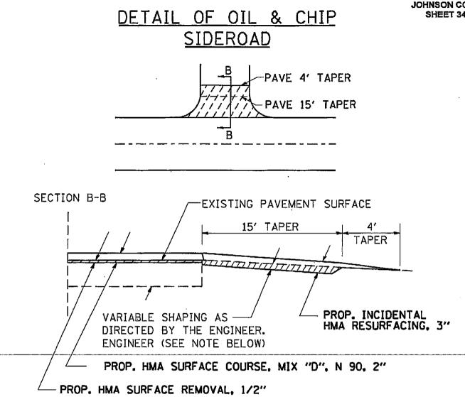
IF EXISTING SUB-BASE IS INADEQUATE, AS DETERMINED BY THE ENGINEER, THE SIDEROADS SHALL BE CORED OUT AND AGGREGATE SUB-BASE, TYPE B SHALL BE PLACED FOR BASE. THE COST OF CORING OUT THE SIDEROAD SHALL BE INCLUDED IN THE COST OF THE AGGREGATE BASE COURSE. IF EXISTING SUB-BASE IS DETERMINED TO BE ADEQUATE, THE AGGREGATE BASE COURSE SHALL BE DELETED AND THE PREPARATION OF THE BASE SHALL BE CONSTRUCTED ACCORDING TO ARTICLE 406.09
