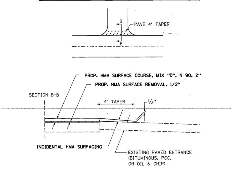
PREPARATION OF EXISTING SURFACE AND ANY EXCAVATION FOR ENTRANCES SHALL BE IN ACCORDANCE WITH ARTICLE 406.09 OF THE STANDARD OF SPECIFICATIONS.
