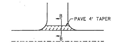
PROP. HMA SURFACE COURSE, MIX "D", N 90, 1 1/2" PROP. HMA BINDER COURSE IL-19.0, N90, 2 1/4" SECTION B-B PROP. HMA SURFACE REMOVAL, 1/2" 4' TAPER 4' TAPER V2" INCIDENTAL HMA SURFACING (THICKNESS EQUAL TO MAINLINE RESURFACING) COR OIL & CHIP)
