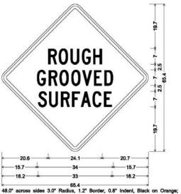
[ROUGH] C 2K 82% spacing; [GROOVED] C 2K 90% spacing; [SURFACE] C 2K 87% spacing;
