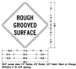
[GROOVED] C 2K 91% spacing; [SURFACE] C 2K 85% spacing;
