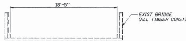
EXISTING TYPICAL BRIDGE SECTION
