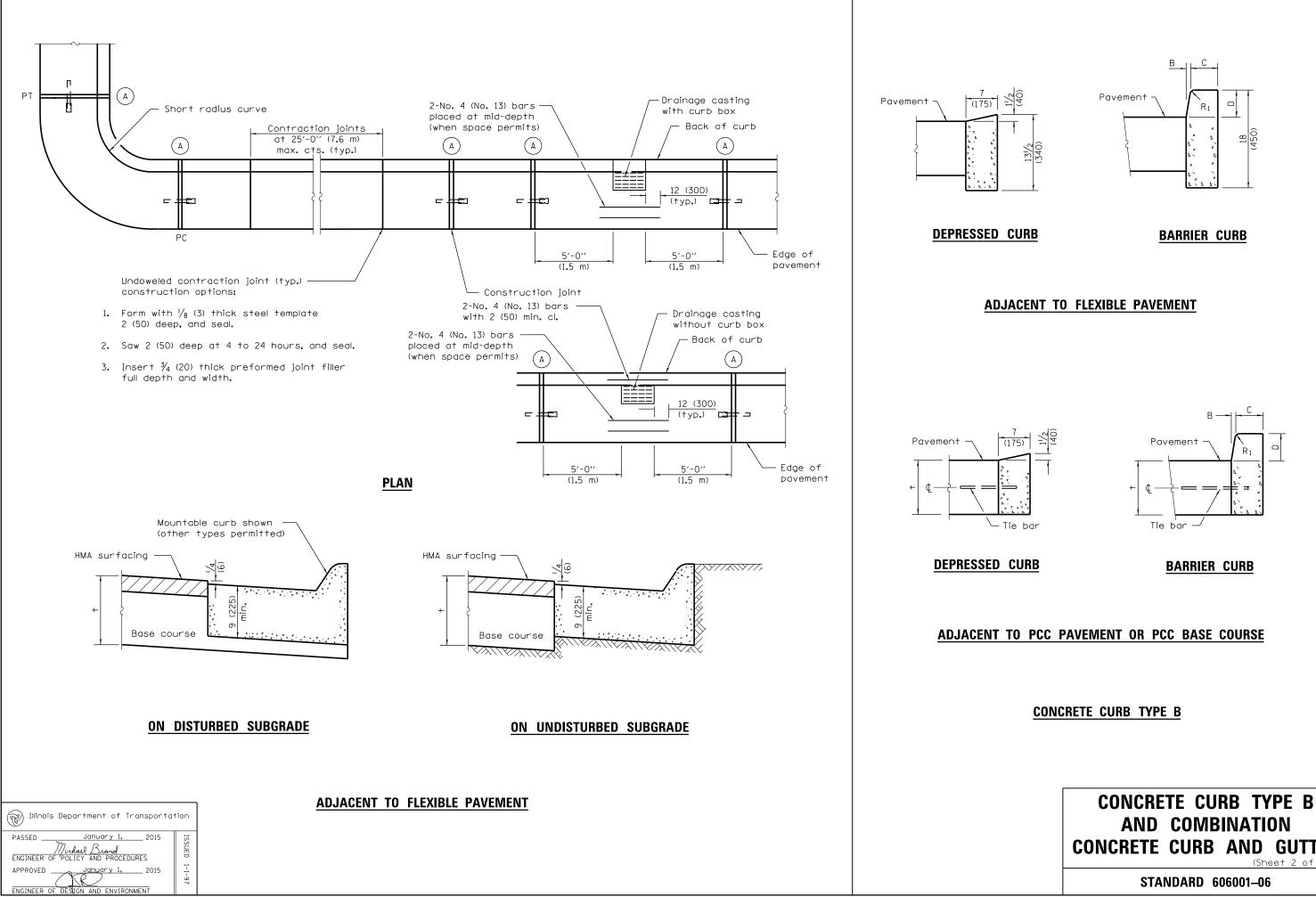
AND COMBINATION **CONCRETE CURB AND GUTTER** (Sheet 2 of 2)
