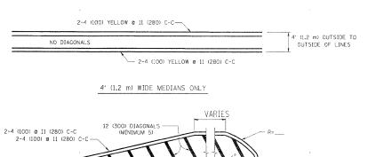
MEDIAN LENGTH FOR MEDIAN LENGTHS WHERE DIAGONAL SPACING CANNOT BE ATTAINED, USE 5 (FIVE) EQUALLY SPACED DIAGONAL LINES.
