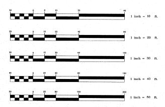
FULL SIZE PLANS HAVE BEEN PREPARED USING STANDARD ENGINEERING SCALES, REDUCED SIZED PLANS MILL NOT CONFORM TO STANDARD SCALES, IN MAKING MEASUREMENTS ON REDUCED PLANS, THE ABOVE SCALES MAY BE USED
