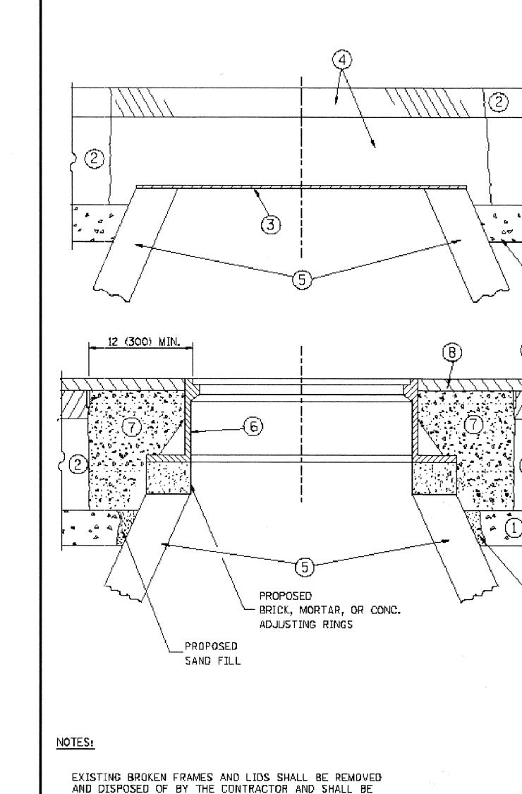
REPLACED AS DIRECTED BY THE ENGINEER. REPLACEMENT
