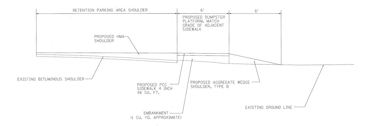
NOTE: PROPOSED HMA SHOULDER IN THE RETENTION PARKING AREA SHOULDER SHALL MATCH THE GRADE OF THE PROPOSED POLYMERIZED HMA SURFACE COURSE, MIX "D", N90
