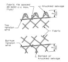
METHOD OF TYING FABRIC TO TENSION WIRES
