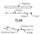
When fence line has a change in direction of 15° or more, a terminal post shall be placed as shown above.
