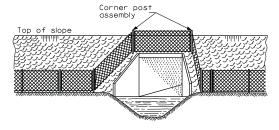
When the width of the culvert makes it necessary to anchor a post to the top of the culvert, a cast iron shoe or other device approved by the Engineer shall be used
