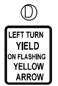
LEFT TURN YIELD ON FLASHING YELLOW ARROW R10-12a 30"X36" SIGN PANEL - TYPE 1 2 REQUIRED
