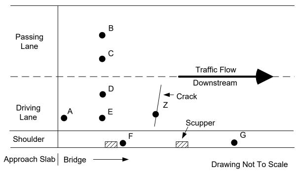
The sample locations are chosen to isolate areas of the deck that have the greatest chloride ion ingress potential and or places where bridge deck wear due to tire traffic is increased. The sample locations are typically isolated to the first 15 feet of the structure to simplify traffic control requirements.
