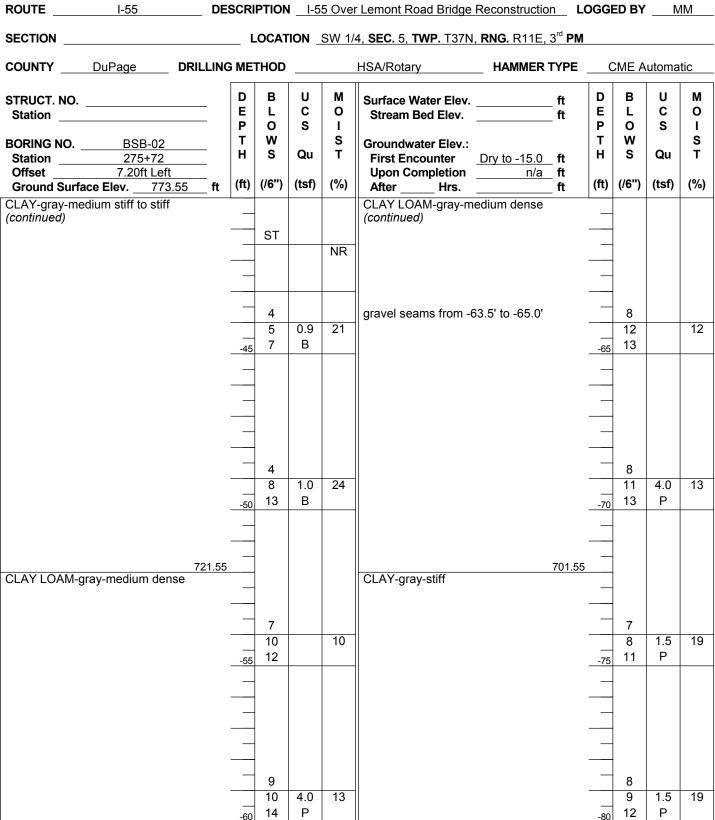
The Unconfined Compressive Strength (UCS) Failure Mode is indicated by (B-Bulge, S-Shear, P-Penetrometer) The SPT (N value) is the sum of the last two blow values in each sampling zone (AASHTO T206), GP-Geoprobe Hand Auger BBS, from 137 (Rev. 8-99)
