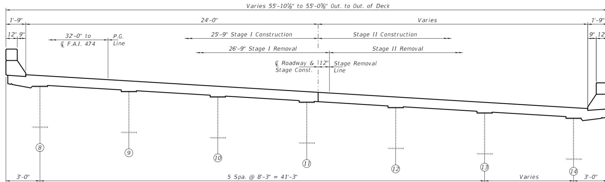
**CROSS SECTION THRU SPAN 2 AT ABUTMENT**
