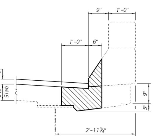
**SECTION THRU CONCRETE REMOVAL & REPLACEMENT AT FLOOR DRAINS**
