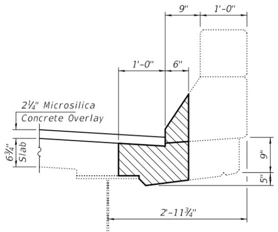
SECTION THRU CONCRETE REMOVAL &
