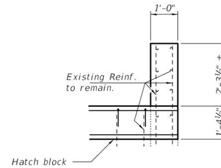
SECTION THRU ABUTMENT AT APPROACH
