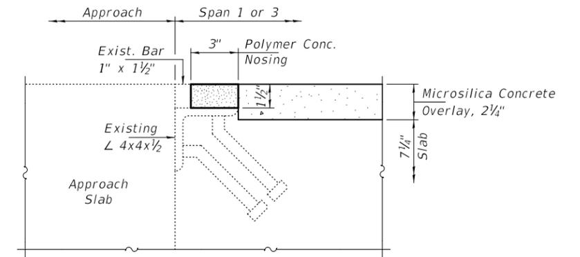
POLYMER CONCRETE NOSING DETAIL
