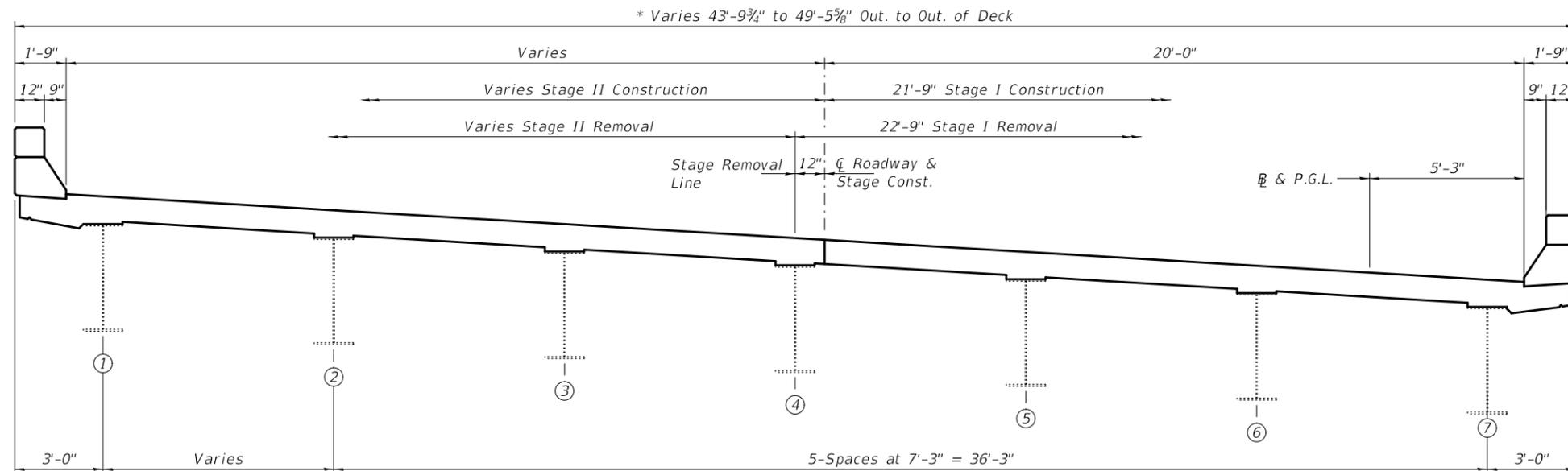
**CROSS SECTION THRU SPAN 2 AT ABUTMENT**
