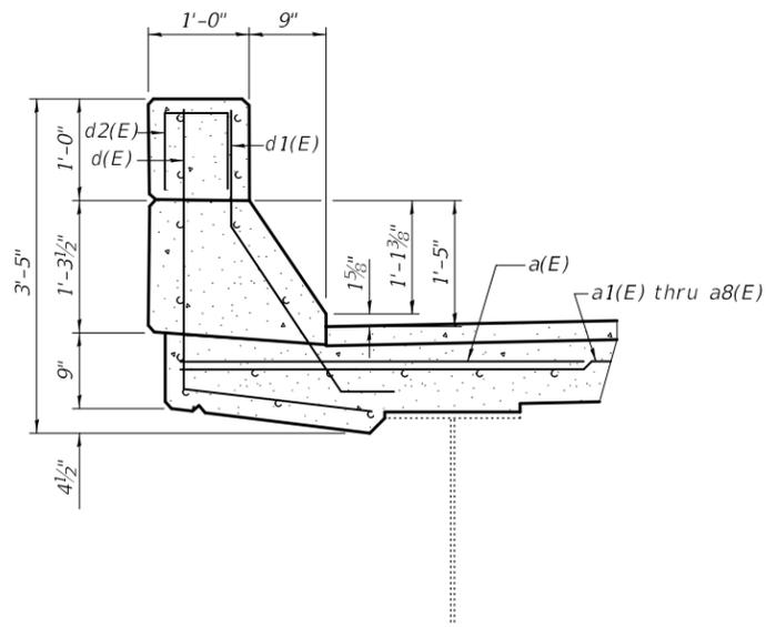
SECTION THRU BRIDGE PARAPET
