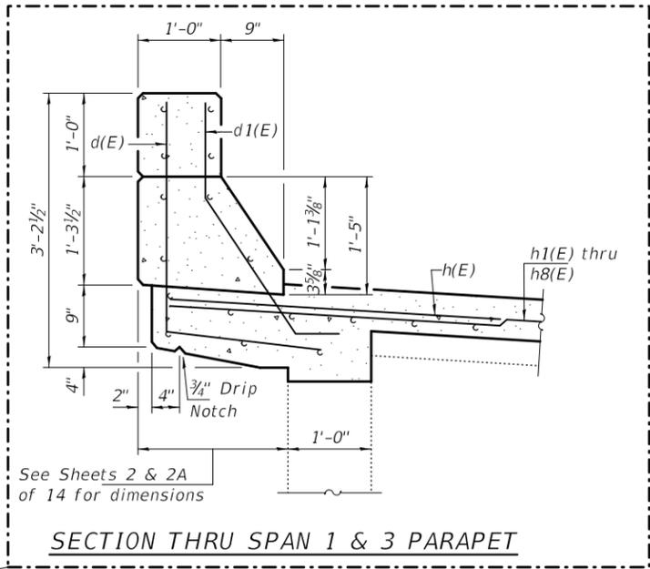
SECTION THRU SPAN 1 & 3 PARAPET
