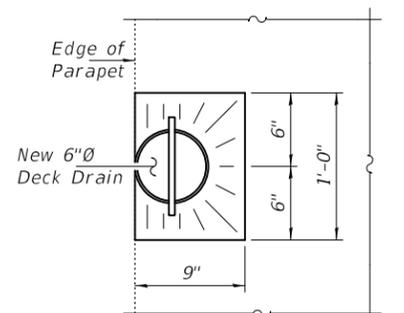
**OVERLAY TREATMENT AT FLOOR DRAINS**
