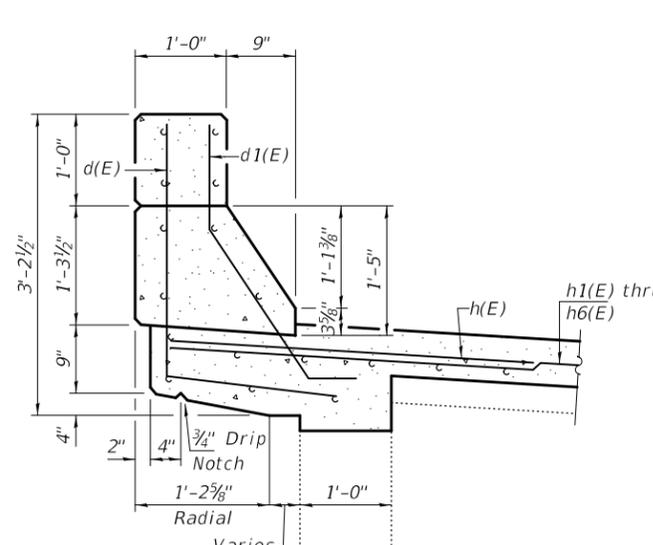
SECTION THRU SPAN 1 & 3 PARAPET
