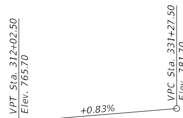
PROFILE GRADE RAMP C (Along E Roadway)
